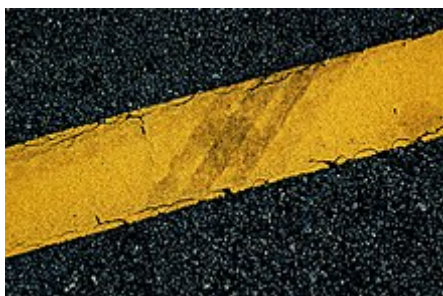
Pigment Yellow 10, a derivative of 1,4-dichloroaniline, is commonly used for yellow road markings in the US.
